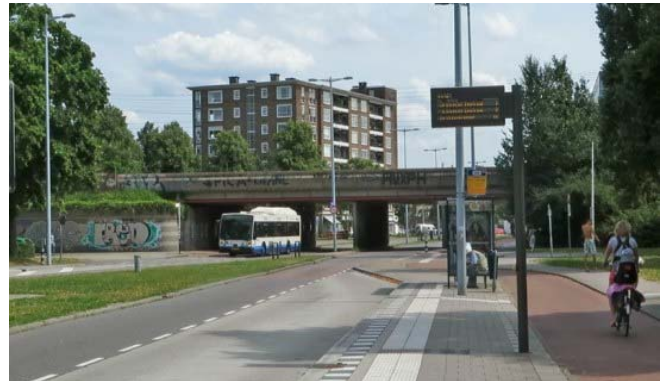
Figure 3. Example showing grouping of bus shelters and pedestrian amenities into pedestrian space and contrasting paving for bike travel way (Europe)
