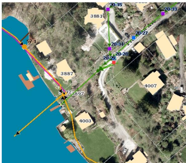
Figure 3: Screen shot of the City of Mercer Island Public Works IGS Utilities Map showing existing stormwater and sanitary sewer utilities.
