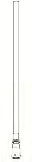
Omni (“whip”)-style antenna 48 to 72 inches high, 1 to 3 inches in diameter
