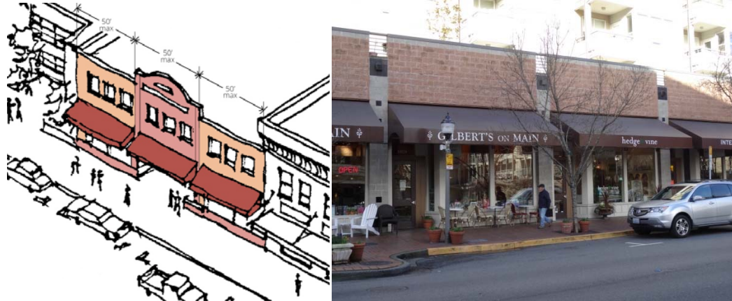
Figure 1213. Minor Façade Modulation examples.
