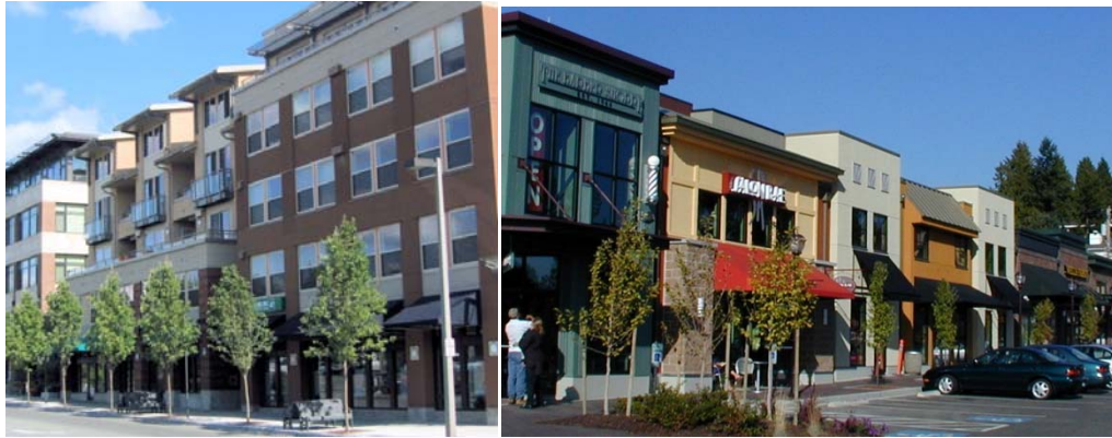
Figure 1011. Façade examples employing building walls with contrasting articulation that make it appear like two or more distinct buildings.
