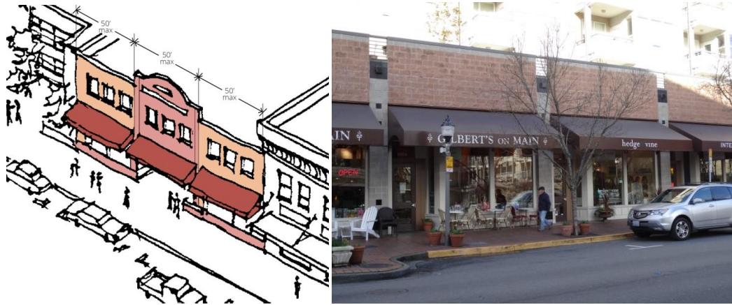
Figure 12. Minor Façade Modulation examples.
