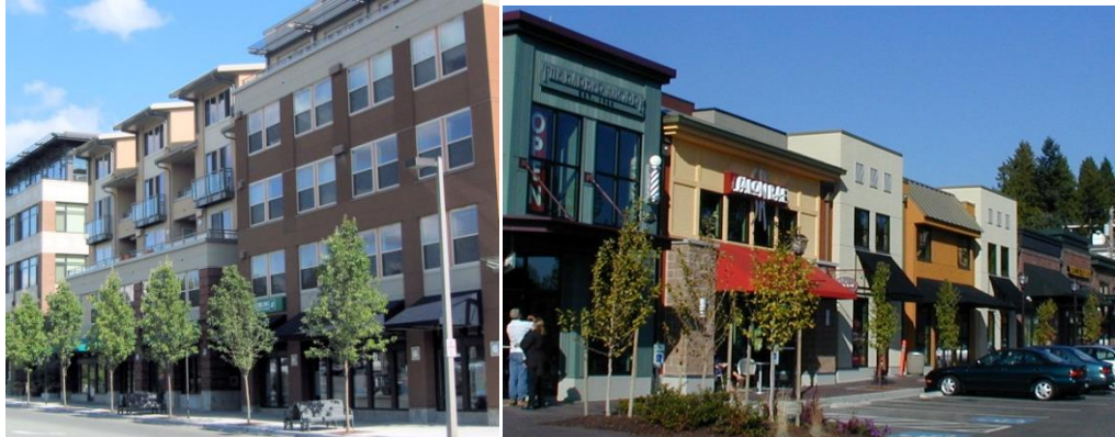
Figure 10. Façade examples employing building walls with contrasting articulation that make it appear like two or more distinct buildings.
