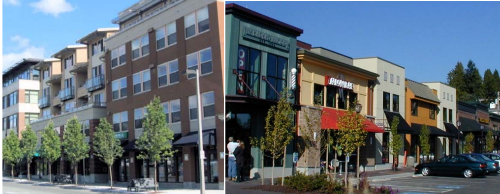
Figure 11. Façade examples employing building walls with contrasting articulation that make it appear like two or more distinct buildings.
