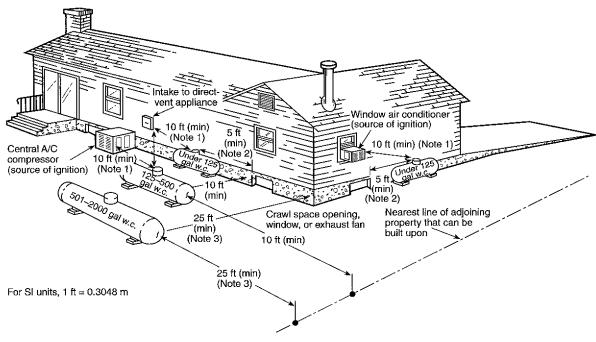
Note 1: Regardless of its size, any ASME container filled on site must be located so that the filling connection and fixed maximum liquid level gauge are at least 10 ft from any external source of ignition (e.g., open flame, window A/C, compressor), intake to direct-vented gas appliance, or intake to a mechanical ventilation system. Refer to 6.3.9.
