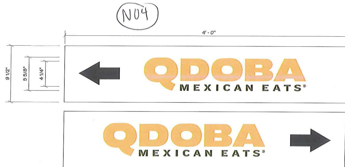
(2) FLAT TENANT PANEL SIGN FACES MANUFACTURED FROM WHITE ACRYLIC WITH DIGITALLY PRINTED GRAPHICS
