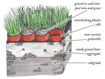
Open-celled grids are concrete grids or rigid, plastic cells that interlock and are pinned in place. The grids or cells are filled with gravel or a mixture of permeable soil/compost and grass that allow water to pass through to the soil underneath. Open-celled grids can support the weight of vehicles and are typically installed in driveways, sidewalks, and patios.
