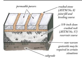
Permeable pavers are interlocking blocks or bricks that come in a variety of materials, colors, and shapes and can be arranged in various patterns. Non-interlocking flagstones or other irregularly shaped pavers can also be installed with 1- to 3-inch gaps or joints between the pavers filled with gravel or a sand/compost mix. The City has prepared design guidelines for residential paver projects (see link in Helpful Resources section of this brochure).
