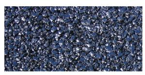
Porous asphalt looks similar to conventional asphalt, but has fewer small particles, which provides open space for water to pass through. Porous asphalt has a rougher surface than conventional asphalt and can be used in low-traffic areas such as residential driveways and sidewalks.
