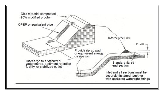
Figure 4.2.4 – Pipe Slope Drain
