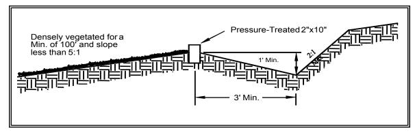
Figure 4.2.5 - Cross Section of Level Spreader
