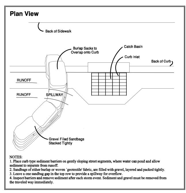
Figure 4.2.10 – Curb and Gutter Barrier
