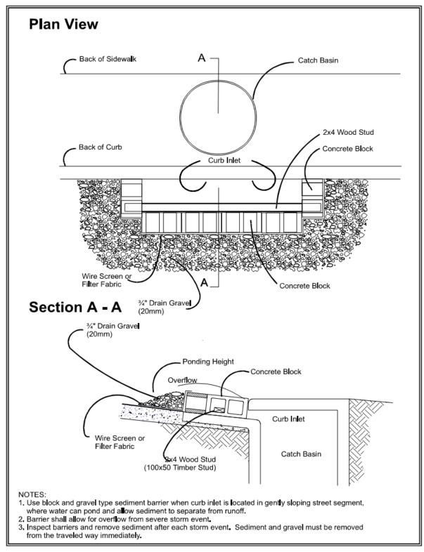
Figure 4.2.9 - Block and Gravel Curb Inlet Protection
