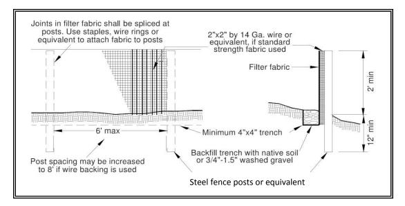
Figure 4.2.12 – Silt Fence
