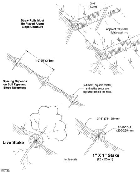
1. Straw roll installation requires the placement and secure staking of the roll in a trench, 3"-5" (75-125mm) deep, dug on contour. runoff must not be allowed to run under or around roll.
