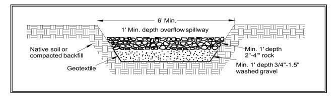
Figure 4.2.17 – Sediment Trap Outlet
