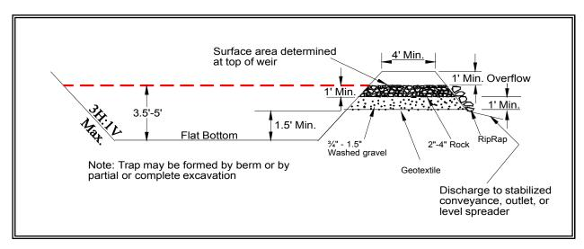
Figure 4.2.16 - Cross Section of Sediment Trap
