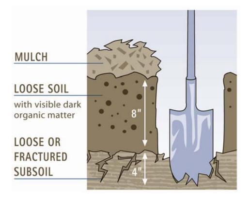
Figure 5.3.3 – Planting bed Cross-Section
