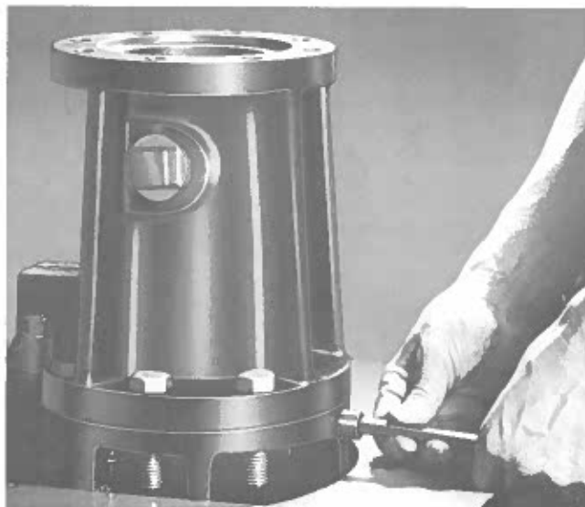
Figure 13 (B) — Removing Vent Plug
